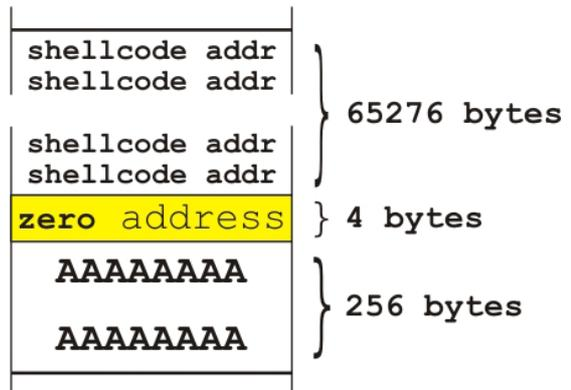
An exploitation is possible but it is not easy. The attacker may use a classical buffer overflow approach<sup>3</sup>, smashing the return address of example program located on the stack. There is only one obstacle – the endless loop. Since **argc[1]** can't contain NULL bytes,
