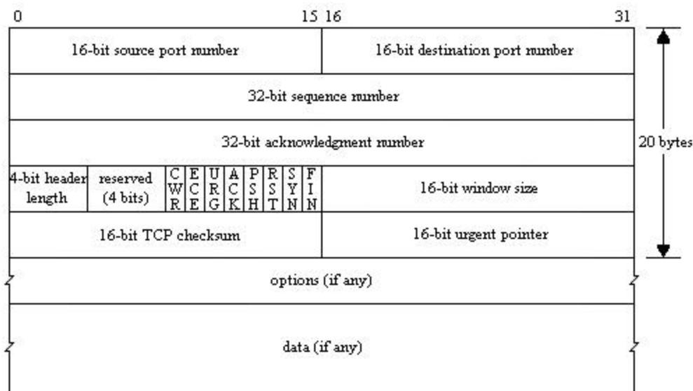
**Figure 1:** TCP header
